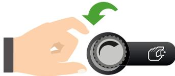
Hold down ON button to release pressure in the device.
