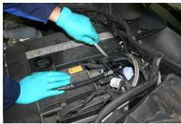
6. Start engine and allow it to idle for several minutes. Delete any error codes that appear. Check fuel system connections for leaks. Replace fuel filter (item No. 13310-12) in the return line of the Injecto-Clean unit.
