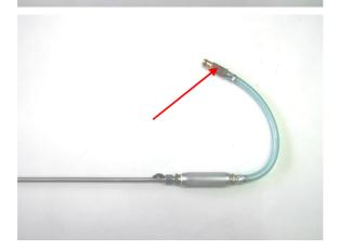
Screw the bayonet nut connector off from the probe. (19 mm open-end wrench)
