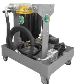
A large, silver and black diesel cleaning pump with a handle and hose, mounted on a grey base with four small wheels. | <p><b>16410 Diesel Clean Pump MDF140</b></p> <p><b>150 l/min</b></p> <p><b>Indicata per serbatoi molto grandi e cisterne grandi fino a 35.000 l</b></p> |
