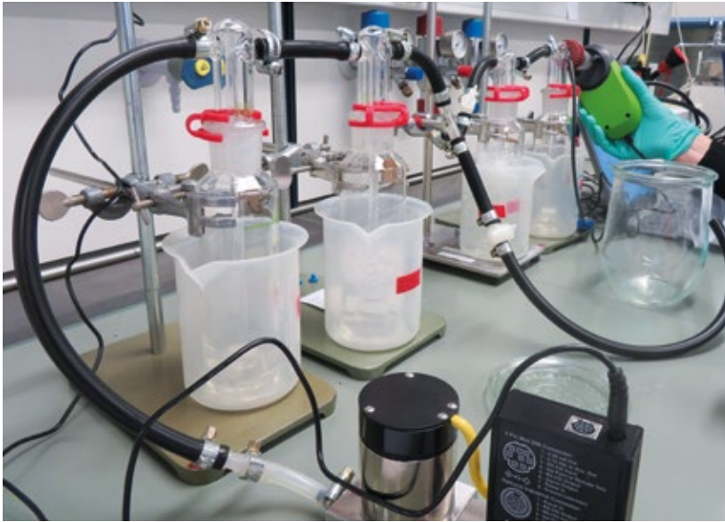
Measurement of the test organism solution with the airco well ® Sensor
