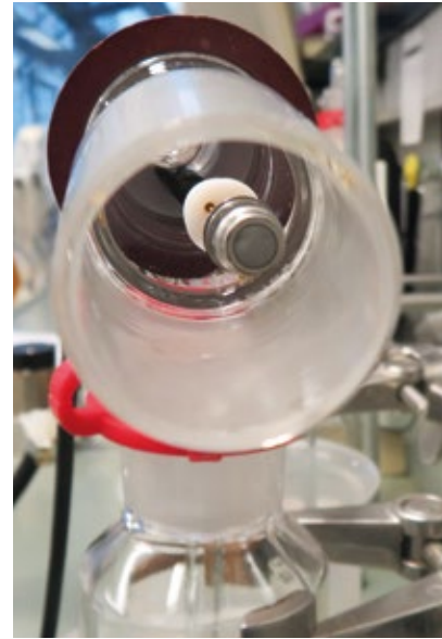
Glass attachment with integrated triple-layer sensor
